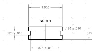
**Stanford Magnets** UNLESS OTHERWISE SPECIFIED, DIMENSIONS ARE IN INCHES TITLE: BLOCK, STEPPED TOLERANCES: FRACTIONAL ± 0.030 ANGULAR: ± 1° SIZE DWG. NO. REV TWO PLACE DECIMAL ± 0.004
