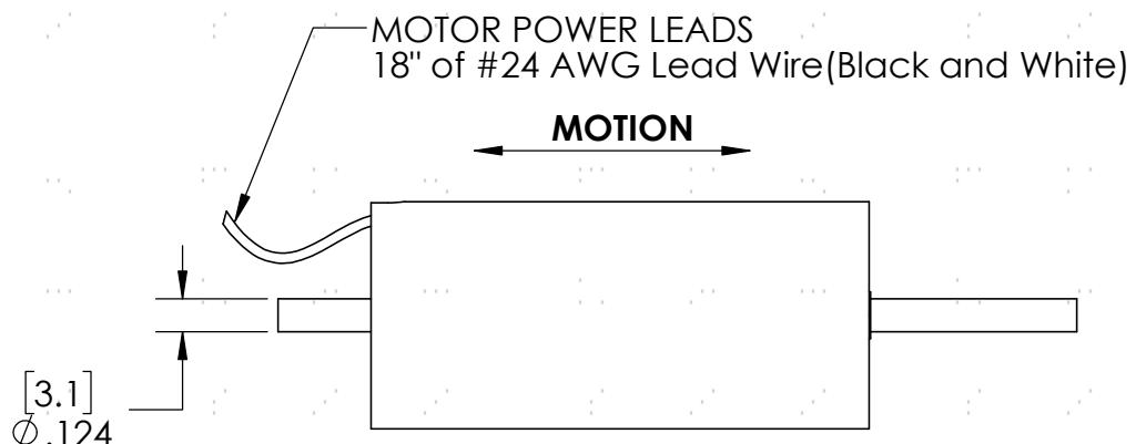
When (+) is connected to WHITE, and (-) is connected to BLACK, the shaft moves away from the leads.
